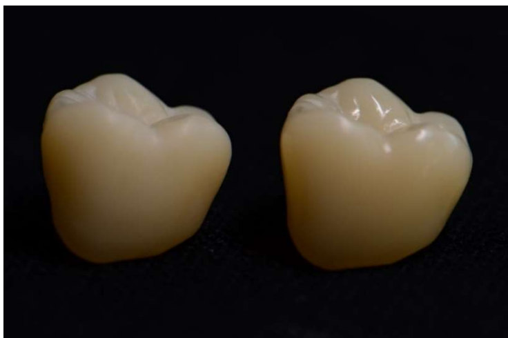
Fig. 15: Tetric CAD: Unpolished, directly after milling (left) and after polishing with Optrapol (right)
