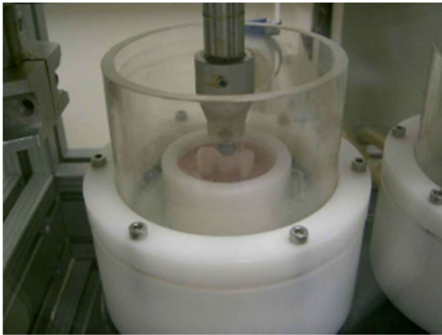
Fig. 9: Willytec chewing simulator
