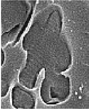
Fig. 8c: Mid-section of Fig. 7a (magnified) showing striations in dissolved area of leucite crystal
