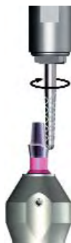
Processing of an abutment with the help of a universal holder (Camlog Biotechnologies AG)
